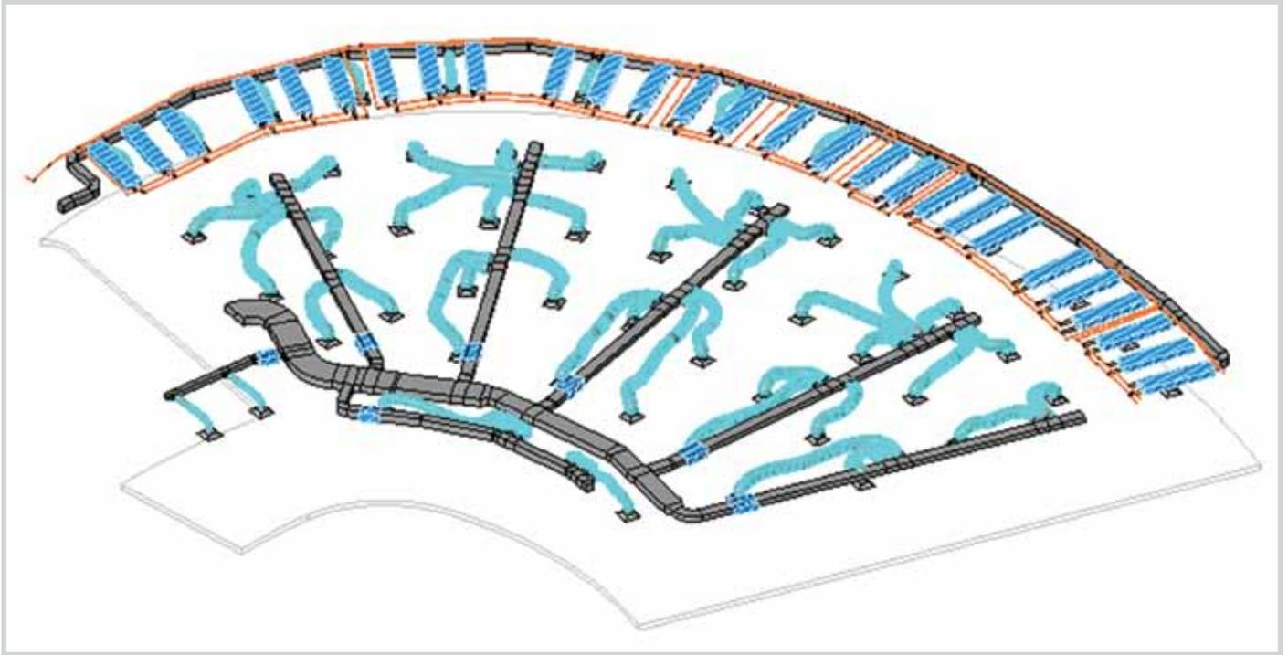
*Mechanical services of a typical floor using Revit® Services*
