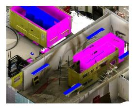
Figure 6.3: Colourised point cloud compared to model (magenta and blue elements)
