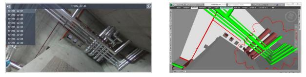
Figure 6.2: On-site photograph (on left) used to update construction model (on right)
