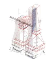
Figure 6.4: Point cloud compared with red wireframe of construction model
