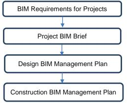
The Design and Construction BIM Management Plans may alternatively be produced as a combined BIM Management Plan.
